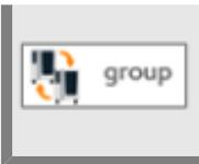
Press the **Group ID** button to assign the unit to a group. By assigning multiple units to a group, these units can be operated from one screen. No more than 10 different groups can be formed.
