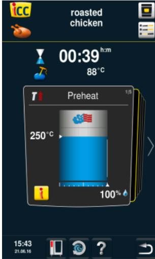
You can open the iCC cockpit by pressing the iCC cockpit button or it will open automatically after 10 seconds. The appliance is pre-heated automatically.
