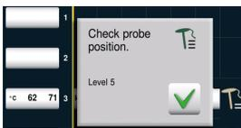
If the probe is inserted incorrectly or if it slips with rolling loads, the following warning appears.
