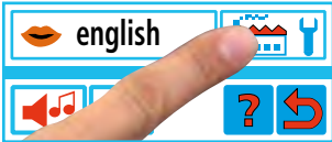
Confirmation, select and hold down "Reset factory default" button. All settings are reset to their factory defaults.
