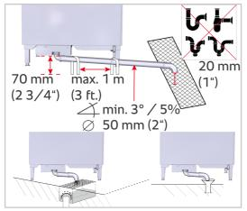
The average height of the wastewater connection is 70 mm [2.76 inch].
