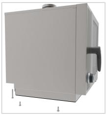
2. Lift the left side wall from below and pull the side wall downwards away from the device.
