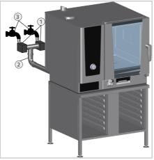
Feed the connections to the device together via Y- or T-piece (Pos. 2) (connection size: 3/4 inch). Connect a check valve between each water tap and the Y- or T-piece (Pos. 1).
