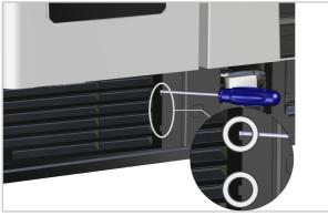
2. Unscrew the blind rivets in the lower left corner.
