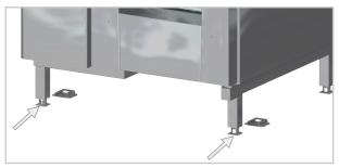
2. Slide the floor device into the foot locks.
