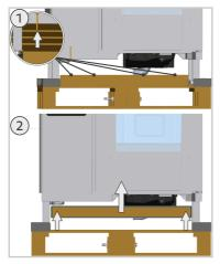
2. Remove the foam rubber next to the device feet from the transport pallet.
