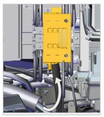
5. Mount the seals and the lock nut on the pipe adapter via the cable.
