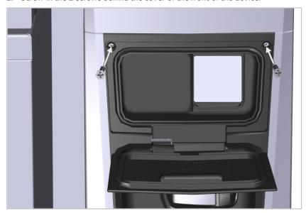
>> The electrical compartment is closed and protected against water and moisture penetration.
