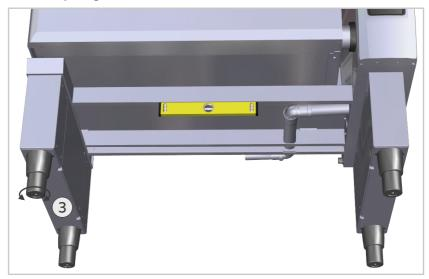
3. Place the spirit level on the bottom of the device and align the device horizontally using the device foot 4.
